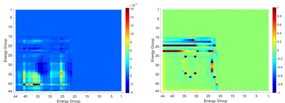
Fig. 5. Covariance contribution from resonance parameters in resolve resonance range for <sup>235</sup>U processed by RXSP and NJOY (left: RXSP, right: the relative difference w/ and w/o self-shielding).
