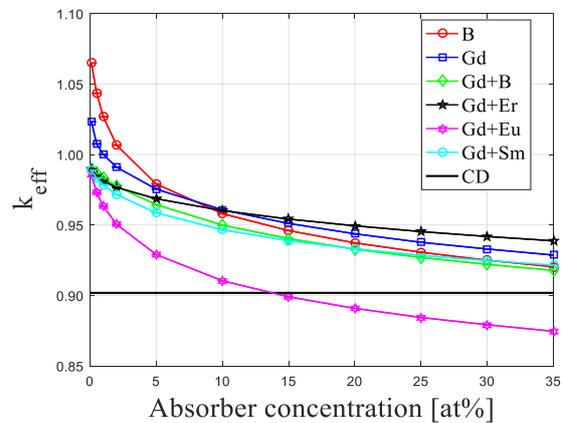
Fig. 4. The comparison of neutron absorption capacity of various materials.
