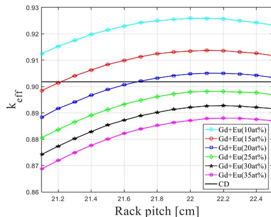
Fig. 5. Optimization of absorber concentration with the reduced rack pitch.
