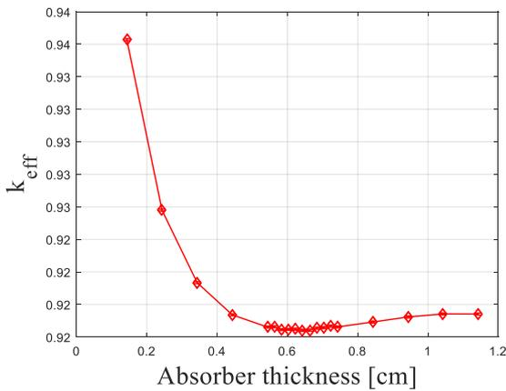
Fig. 2. The  $k_{eff}$  with the annular cylinder type neutron absorber thickness.
