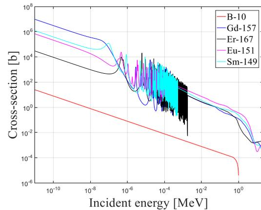
Fig. 3. The neutron absorption cross section of selected candidates for neutron absorber material.
