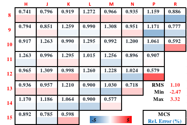
Fig. 4. The Normalized Radial Assembly Power Distribution compared with Measured at MOC (6 GWd/MT).
